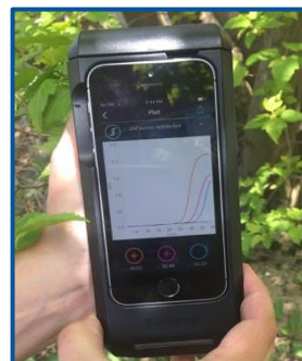
Fig 3. The Biomeme two3™ thermocycler displaying qPCR results.
